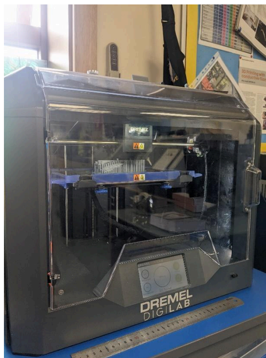
Figure 14.5. The rocket model was printing.
