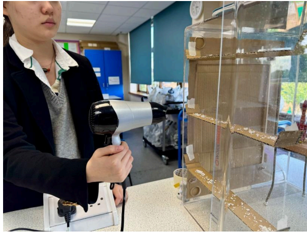
Figure 16.5. Creating wind and turbulence by using a hairdryer.
