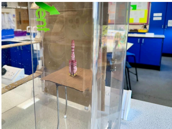
Figure 16.4. The rocket model was mounted on a tripod platform made of gauze and cardboard.
